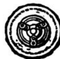
Stand for proof of B.L. plain and R.L. screw percussion fuses, Mark I.
